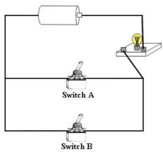
d) If both switches are turned on, the bulb will be  $\dots$
