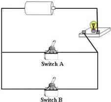
b) If Switch A is turned on and Switch B is turned off, the bulb will be ...
