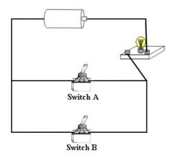
a) If Switch A and Switch B are both turned off, the bulb will be ...
