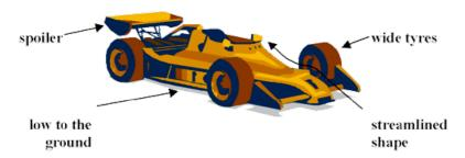
What helps a racing car go fast? Explain how these parts of the racing car can help it go faster.
