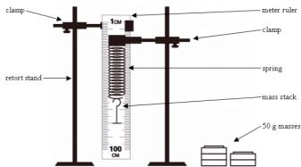
a) What is the reading for the spring length on the meter ruler before the mass stack is attached?
