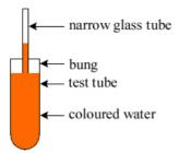
Susie made a water thermometer. She tested her thermometer at different temperatures.
