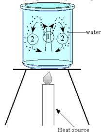
A glass beaker is filled with water and some glitter is dropped into it. The movement of the glitter shows how liquid moves when it is heated.
