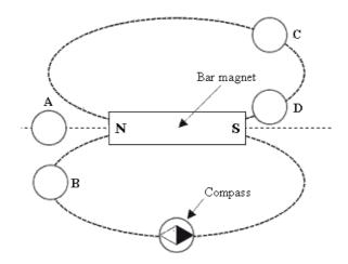
Peter was working out a line of magnetic force using a compass as an indicator.
