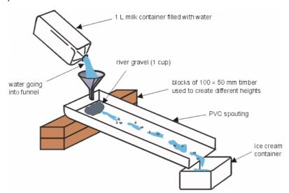
NOTE: We used  $100 \times 50$  mm timber offcuts, to make the different heights. We used no blocks (for 0 cm), 2 blocks (which is approximately 10 cm), and 4 blocks (which is approximately 20 cm).
