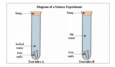
Information: The boiling of water removes dissolved gases.
