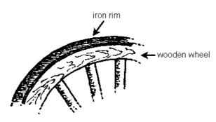
Years ago, wooden wheels had iron rims fitted. To fit the iron rim, it was heated, then put around the wooden wheel and allowed to cool.
