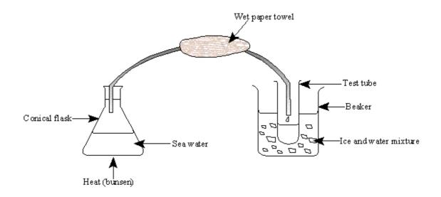
This apparatus was set up to separate and collect fresh water from sea water. There are three changes of state (e.g., solid  $\rightarrow$  liquid) occurring in this diagram. What are these changes, and where are they occurring?
